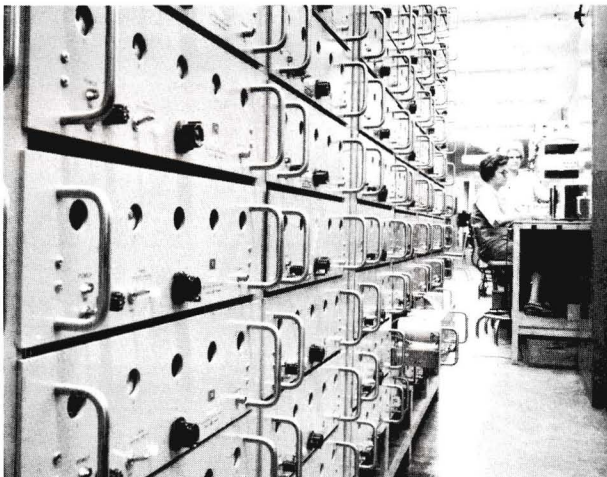
In one of numerous tests, all Model 5245, 5247, and 5248 crystal oscillator assemblies are operated and observed for two weeks to determine aging rates.
